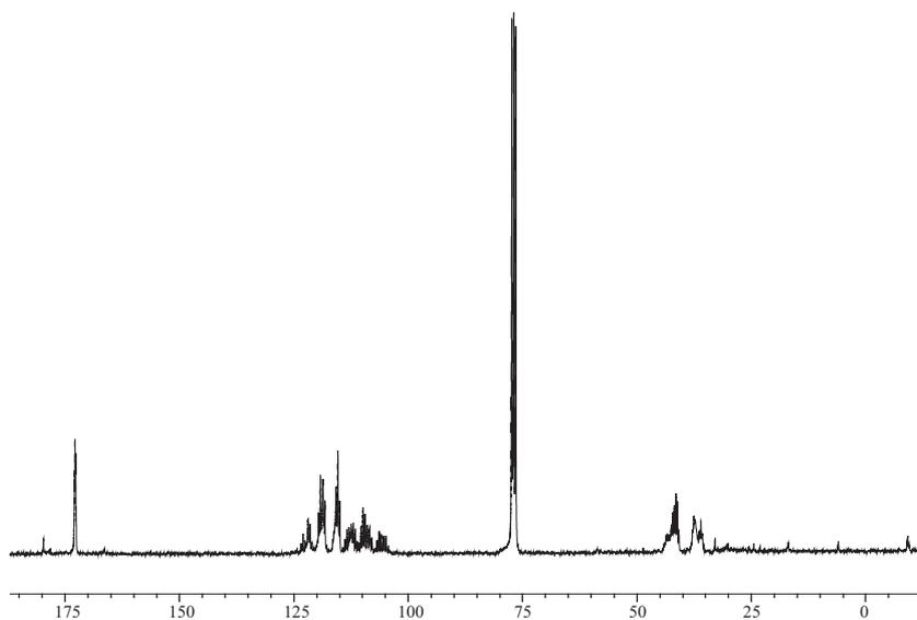
Fig. 3.  $^{13}\text{C}$  NMR spectrum of 3,3,5,5,7,7,8,8,9,9,10,10,10-tridecafluorodecanoic acid (recorded in  $\text{CDCl}_3$ ).
