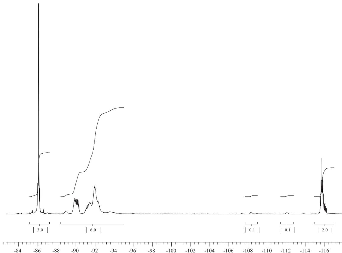
**Fig. 1.** Expansion of the  $-82$  to  $-118$  ppm zone of the  $^{19}\text{F}$  NMR spectrum of the total product mixture of the radical telomerization of VDF with  $\text{C}_2\text{F}_5\text{I}$  initiated by *tert*-butyl peroxyphthalate for a three fold excess of VDF about  $\text{C}_2\text{F}_5\text{I}$  (recorded in  $d_6$ -acetone).
