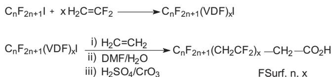
Two surfactants were synthesized: C<sub>2</sub>F<sub>5</sub>(CH<sub>2</sub>CF<sub>2</sub>)<sub>2</sub>CH<sub>2</sub>COOH and C<sub>4</sub>F<sub>9</sub>(CH<sub>2</sub>CF<sub>2</sub>)<sub>2</sub>CH<sub>2</sub>COOH. In the former case (*n* = *x* = 2), the reaction led to a PFOA alternative of similar C<sub>8</sub>-chain length. Each step is described hereafter.
