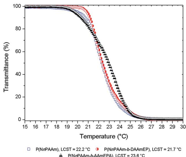
**Fig. 6** Plot of transmittance as a function of the temperature for aqueous solution (5 g L<sup>-1</sup>) of poly(*N-n*-propylacrylamide)-*b*-(diethyl 2-(acrylamido)ethylphosphonate)) (P(*Nn*PAAm-*b*-DAAmEP)) and poly(*N-n*-propylacrylamide)-*b*-(2-(acrylamido)ethylphosphonic acid)) (P(*Nn*PAAm-*b*-AAmEPA)). Ramp temperature: 0.2 °C min<sup>-1</sup>, from 15 to 30 °C.
