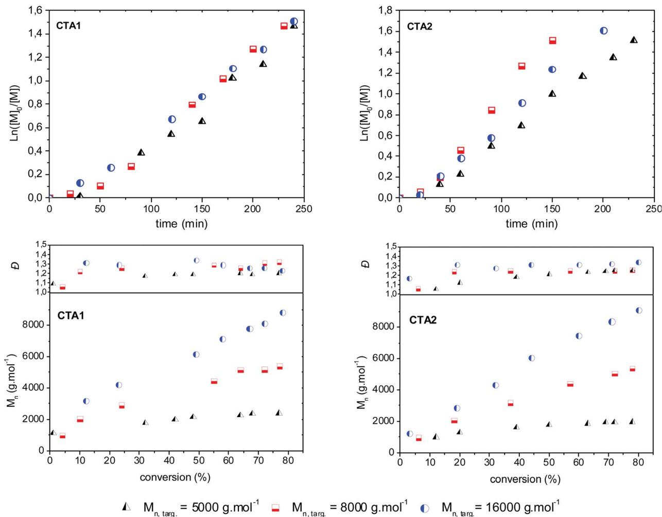
**Fig. 1** Kinetic plots and evolution of the molecular weight with conversion for RAFT polymerization of DAAMeP using CTA1 and CTA2 as a chain transfer agent.
