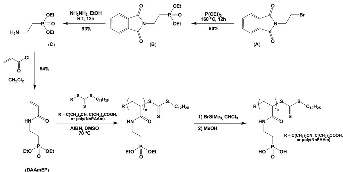
**Scheme 1** Synthetic pathway for the synthesis and RAFT polymerization of the diethyl 2-(acrylamido)ethylphosphonate monomer (DAAmEP) using three different chain transfer agents 2-cyano-2-propyl dodecyl trithiocarbonate (CTA1), 2-(dodecylthiocarbonothioylthio)-2-methylpropionic acid (CTA2), and P(*Nn*PAAm).
