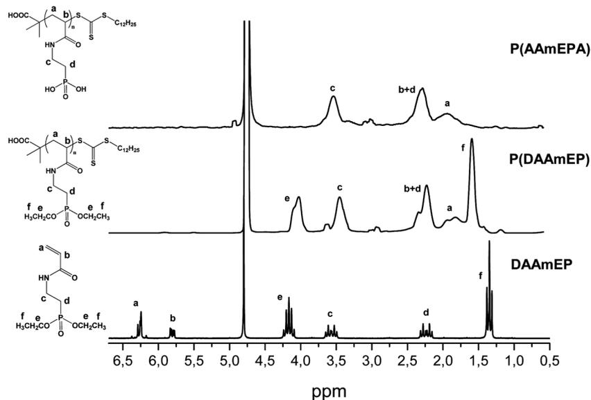
**Fig. 2**  $^1\text{H}$  NMR spectrum of diethyl 2-(acrylamido)ethylphosphonate (DAAmEP), poly(diethyl 2-(acrylamido)ethylphosphonate) (P(DAAmEP)), and poly(2-(acrylamido)ethylphosphonic acid) (P(AAmEPA)) in deuterated water.
