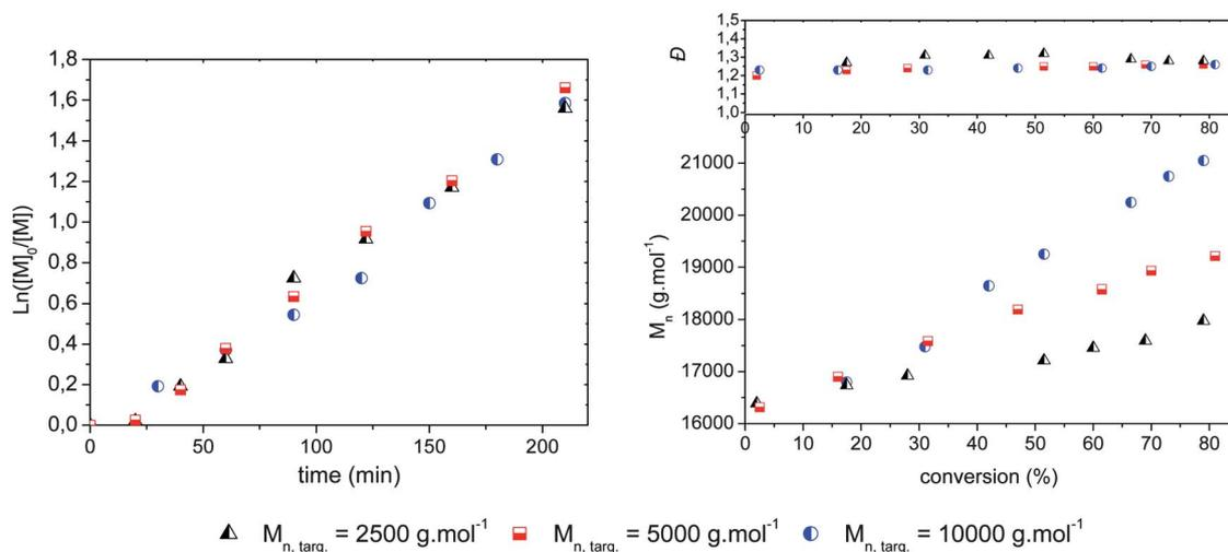
**Fig. 3** Kinetic plots (left) and evolution of molecular weight with conversion (right) for the RAFT polymerization of diethyl 2-(acrylamido)ethylphosphonate (DAAmEP) using poly(*Nn*-propylacrylamide) (P(*Nn*PAAm)) as a macro-chain transfer agent ( $M_n = 9900\text{ g mol}^{-1}$ ).  $M_{n,\text{targ}}$  corresponds to the targeted molecular weight for the phosphonated block at 80% conversion.
