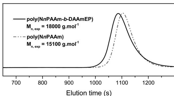
**Fig. 5** Size exclusion chromatograms of the poly(*N*-*n*-propylacrylamide) (*P(NnPAAm)*) macro-chain transfer agent (Table 1, entry 7) and the poly(*N*-*n*-propylacrylamide)-*b*-(diethyl 2-(acrylamido)ethylphosphonate)) (*P(NnPAAm-b-DAAmEP)*) diblock copolymer (Table 1, entry 8) (DMAc eluent + LiCl 0.1% weight at 0.8 mL min<sup>-1</sup>, with PS standards at 50 °C).
