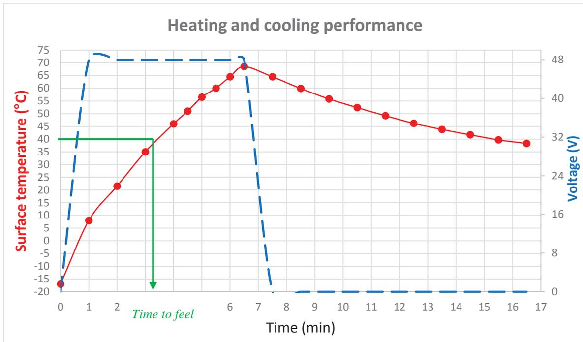
Figure 6: Heating behavior of thermoplastic heating panels
