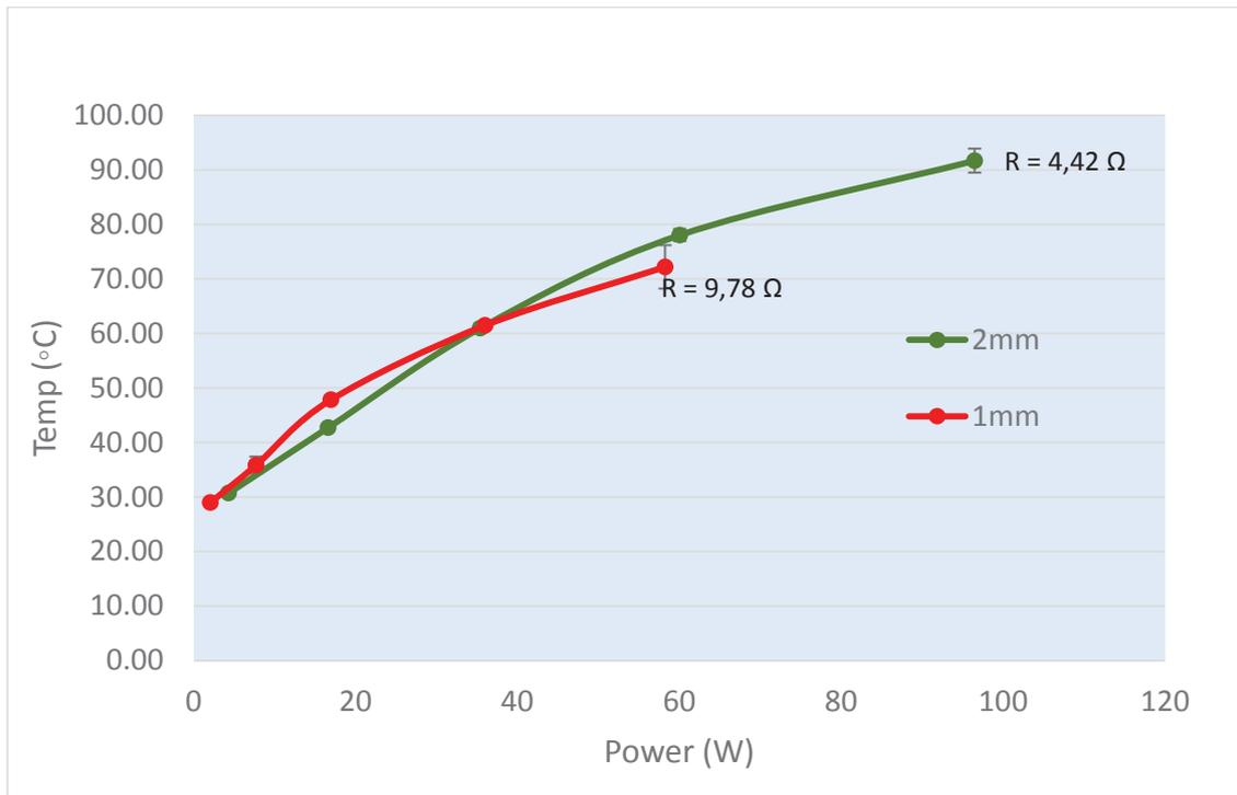
Figure 7: Influence of the sheet thickness on the heating performance
