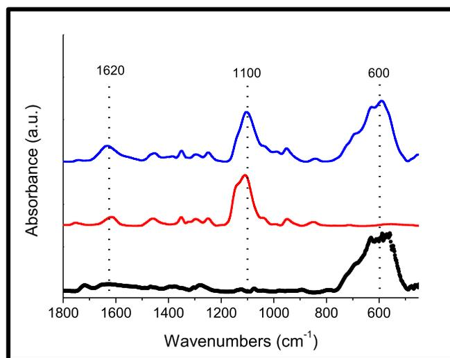
Fig. 3. Infrared spectrum of the uncoated NPs (black), free molecules PO-PEG-COOH (red) and  $\gamma\text{Fe}_2\text{O}_3$ @PO-PEG-COOH NPs (blue). The spectra were normalized with the Fe–O vibration band at 600 cm<sup>-1</sup>.
