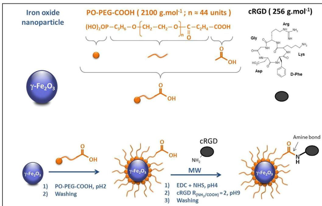
Fig. 1. Schema of the different steps for the synthesis of nanoplatforms.
