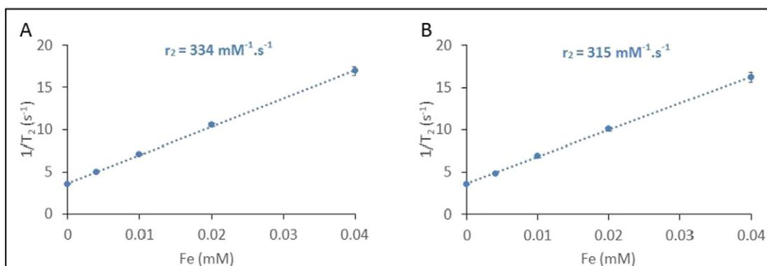
**Fig. 5.** *In vitro* transversal relaxivities measurements at 11.7 T of  $\gamma\text{Fe}_2\text{O}_3$ @PO-PEG-COOH (A) and  $\gamma\text{Fe}_2\text{O}_3$ @PO-PEG-cRGD (B).
