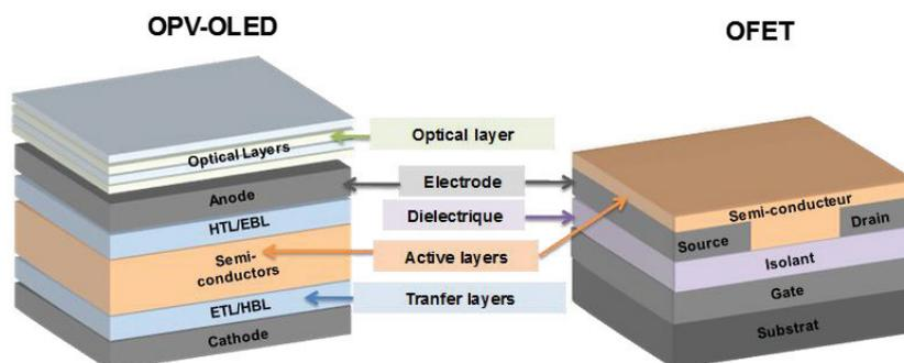
Fig. 3: SPECIFIC POLYMERS – Thin layer materials for optoelectronic devices
