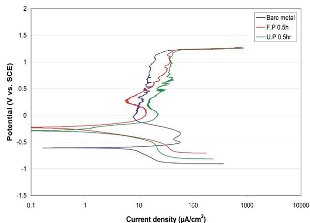
Fig. 1 Potentiodynamic polarization curves for layers formed at 0.5 h with undecenyl and fluoro-phosphonic acids in  $\text{NaClO}_4$  solution
