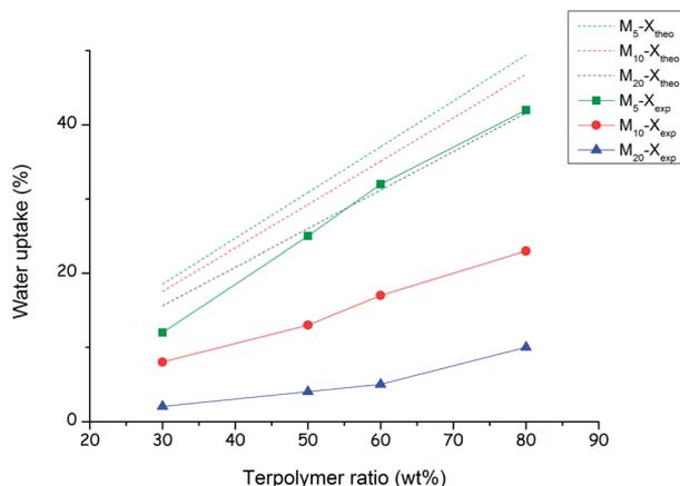
Fig. 7 Evolution of the water uptake vs. the content of fluorophosphonate terpolymer for the  $M_5-X$ ,  $M_{10}-X$  and  $M_{20}-X$  membranes.
