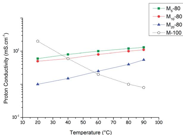
Fig. 9 Average conductivity versus temperature in immersed conditions for the M100, M<sub>5</sub>-80, M<sub>10</sub>-80 and M<sub>20</sub>-80 membranes.
