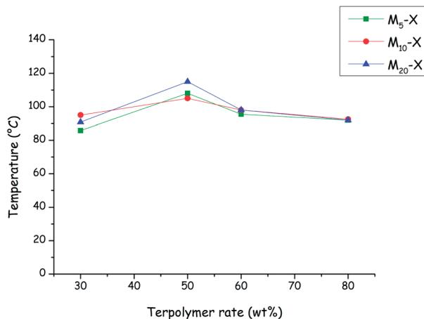
Fig. 6 Evolution of  $T_g$  vs. the content of fluorophosphonate terpolymer for the membranes  $M_5$ ,  $M_{10}$  and  $M_{20}$  after acidification.
