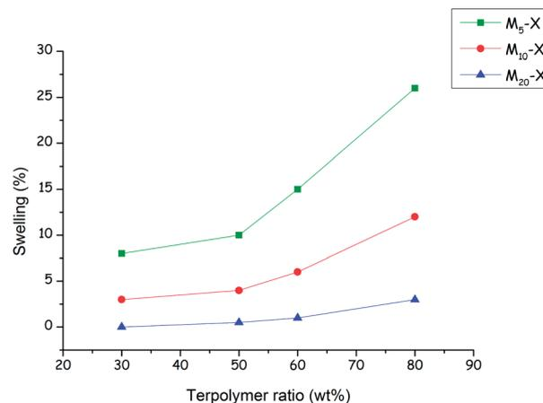
Fig. 8 Evolution of the swelling rate (%) vs. the content of fluorophosphonate terpolymer for the  $M_5$ ,  $M_{10}$  and  $M_{20}$  membranes.
