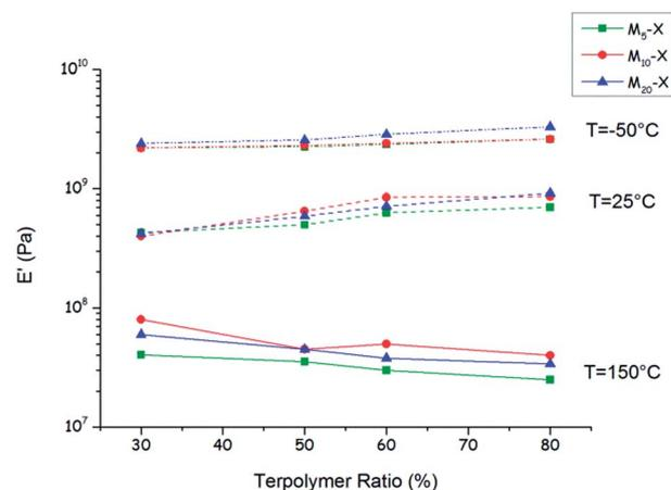
Fig. 12 Storage modulus evolution versus the content of phosphonate terpolymer at  $-50$ ,  $25$  and  $150\text{ }^\circ\text{C}$  for the M<sub>5</sub>-X, M<sub>10</sub>-X and M<sub>20</sub>-X membranes.
