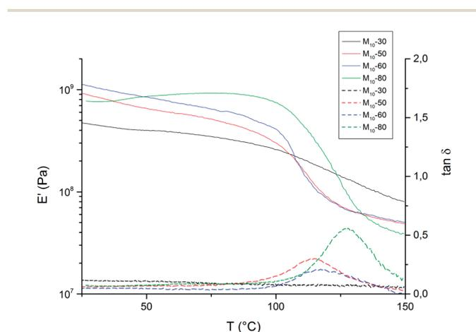
Fig. 11 Storage modulus (—) and  $\tan \delta$  (---) evolution versus temperature for the M<sub>10</sub>-30, M<sub>10</sub>-50, M<sub>10</sub>-60 and M<sub>10</sub>-80 membranes.
