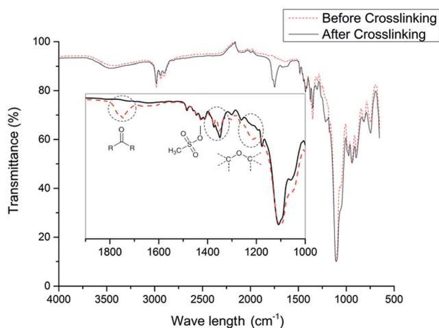
**Fig. 3** FTIR spectrum of poly[(CTFE-*alt*-EVE)<sub>0.9</sub>-CO-(CTFE-*alt*-VBMS)<sub>0.1</sub>] before and after crosslinking.
