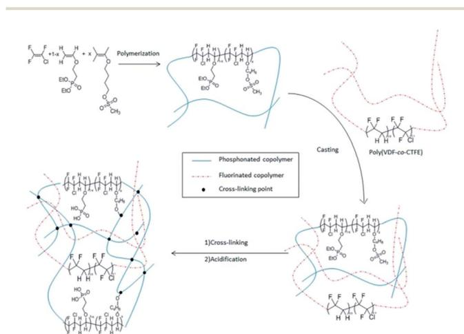
Fig. 5 Schematic representation of procedure to obtain pseudo semi-IPN membrane comprising crosslinked poly[(CTFE-*alt*-DEVEP)-co-(CTFE-*alt*-VBMS)] and poly(VDF-co-CTFE).
