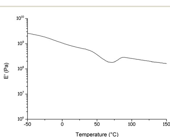
Fig. 10 Storage modulus versus temperature of M-0 performed at 1 Hz and 2 °C min<sup>-1</sup>.
