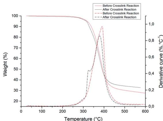
Fig. 2 TGA analyses of poly[(CTFE-*alt*-EVE) $_{0.9}$ -*co*-(CTFE-*alt*-VBMS) $_{0.1}$ ] before and after the crosslinking reaction.
