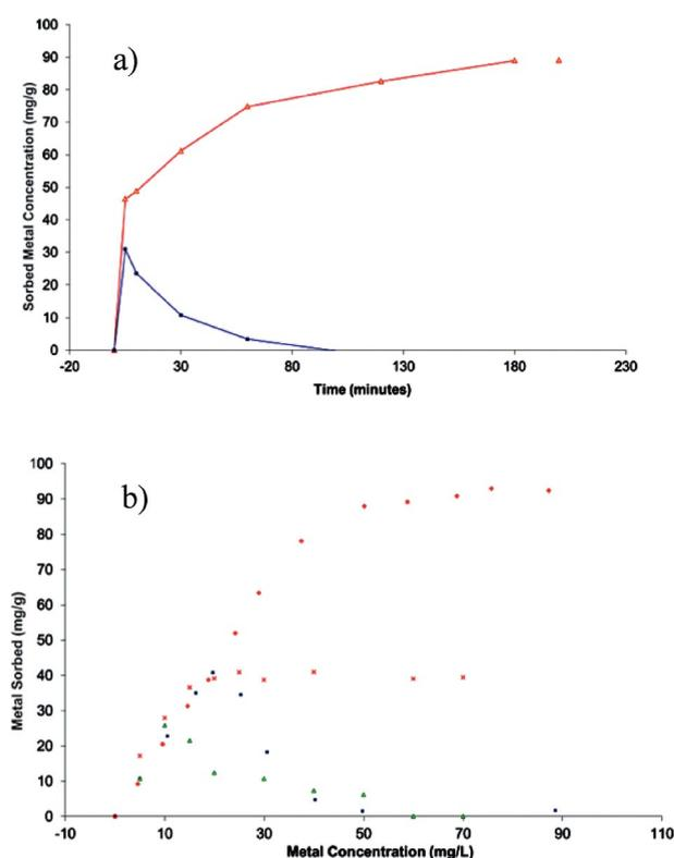
Figure 5. (A) Effect of stirring time on the sorption of Ce<sup>3+</sup> (red) and Sr<sup>2+</sup> (blue) onto SiP-TiO<sub>2</sub> (ANa). Initial Sr sorbance was reversed within the first 15 min. (B) Sorption isotherm of Ce (red diamonds), Sr (blue squares), and Cs (green/yellow triangles) solution on SiP-TiO<sub>2</sub> (ANa). The red x symbols represent the Na<sup>+</sup> released by the SiP-TiO<sub>2</sub> (ANa) as it absorbed the other metals.
