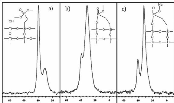
Figure 4.  $^{31}\text{P}$  MAS-NMR spectra of (a) SiP-TiO<sub>2</sub> BH, (b) AH, and (c) ANa. The structural insets represent the possible structure of the majority of the surface SiP for that particular NMR spectrum. The peak at  $\delta = 40$  ppm is believed to be unhydrolysed SiP, whereas the peak at  $\delta = 30$  ppm is the hydrolysed analogue. The sharper version of the 30 ppm peak in spectrum (c) is due to presence of sorbed Na<sup>+</sup> ions.
