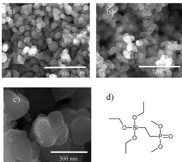
Figure 1. ESEM images of SiP-TiO<sub>2</sub> (a) before, and (b and c) after hydrothermal treatment. (d) Depiction of the SiP functionality.
